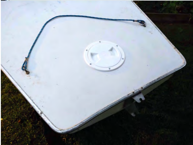
Pictures above show the ports that were installed in the Sunfish boats that did not have them. The ports allow better water drainage from the hulls and let them dry out after taking on any water, thus lighter. All the work was done by Master Boat Improver Dale Sturm and his apprentice.
